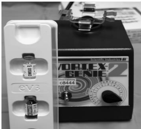
Figure 21 Onyx components: dimethyl sulfoxide (DMSO) vial, Onyx vial, and shaker. The Onyx needs to be shaken for ~20 minutes before use.
